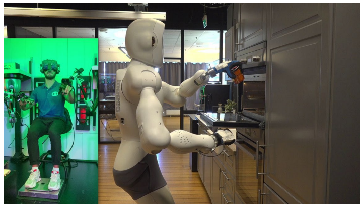
Fig. 1. Operator controls a humanoid avatar robot and receives multisensory feedback including vision, audition, temperature, force, and tactile cues.
