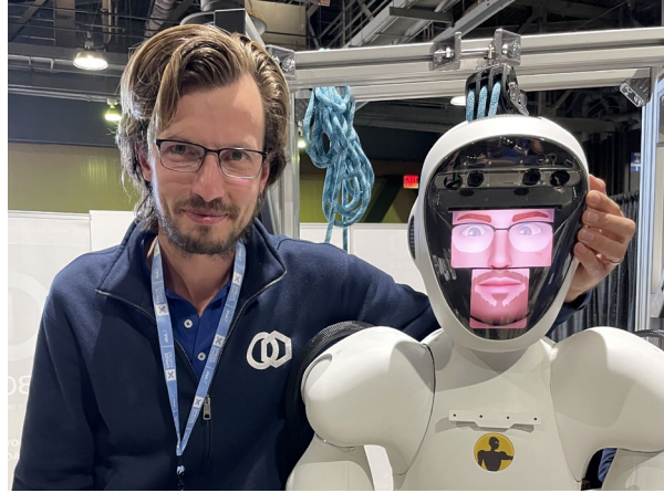
Fig. 2: The humanoid avatar depicts the animated face of the operator in real time. This allows the people in the remote environment to identify the operator, read the operator's facial expressions and follow the eye gaze of the operator.
